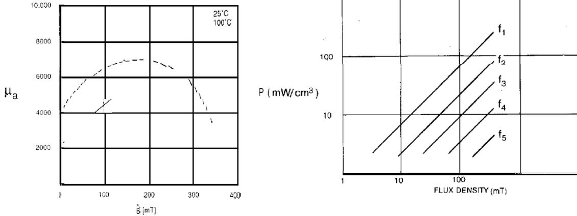
Figure 16-1. Amplitude Permeability vs Flux density
