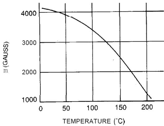
Figure 15-3. Flux Density vs Temperature
