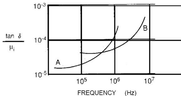
**Figure 15-1. Loss Factor vs Frequency for 2 Materials**
